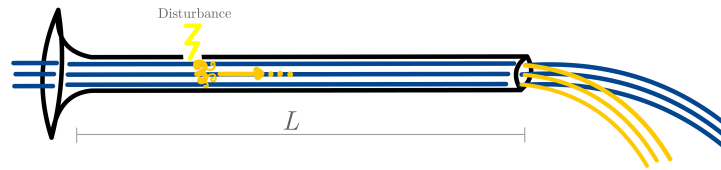
Figure 2: Experimental setup of Hof's experiment [9]. It consists of a pipe connected to a fluid reservoir (to the left) of length L with a controlled access to introduce a disturbance to the fluid flow. A binary measurement of the death or survival of a puff is done by measuring the fluid's outflow velocity at the pipe's outlet.
