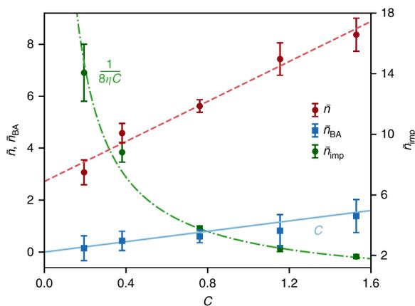
Figure 8: The observed power spectral density is proportional to a sum of various occupation numbers  $n$ . This graph presents the individual components:  $\bar{n}$  is the occupation number of the observed oscillator, the signal.  $\bar{n}_{\text{imp}}$  is the shot noise and  $\bar{n}_{\text{BA}}$  is the noise due to heating back-action. Taken from [6].
