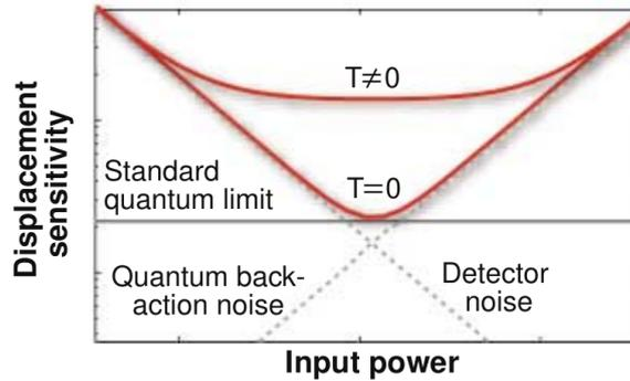
Figure 1: The relationship between displacement sensitivity and laser power in an interferometer; we observe two competing effects: increasing laser strength improves signal-to-noise ratio, but on the other hand introduces quantum back action. Taken from [1].
