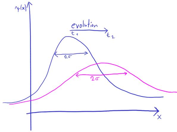
Figure 3: Free evolution of a Gaussian wavepacket. Its mean value moves uniformly in one direction (according to its group velocity) while its half-length increases.
