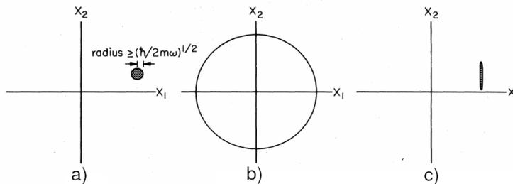
Figure 2: Various modes of measurement for two conjugate variables. a) Amplitude and phase measurement, where we measure both coordinates  $X_1$  and  $X_2$ . In the case of minimum errors, we obtain an error circle. b) Photon counting, where we measure  $N$ , but ignore phase. The result is a circle. c) BAE measurement, where we minimise the uncertainty of  $X_1$  at the expense of  $X_2$ . Taken from [1].
