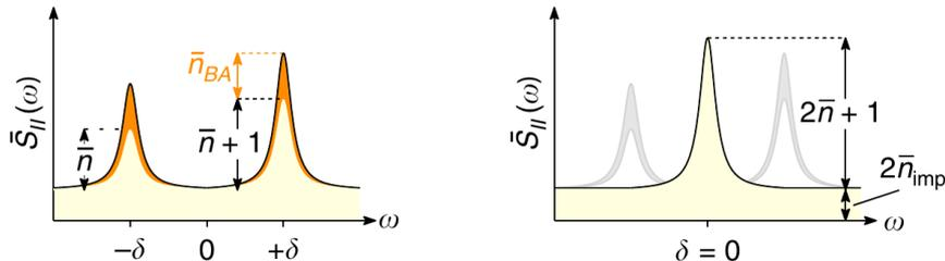
Figure 7: Observed power spectral density from eq. 36. In the left picture we observe two sidebands and a QBA noise contribution in orange. In the right picture we have set  $\delta = 0$ , thus eliminating QBA and uniting the two sidebands. Taken from [6].
